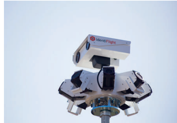
The IdentiFlight stereo camera system detects as well as identifies bird species. It allows for a targeted mitigation effort by curtailing the relevant wind turbine.
