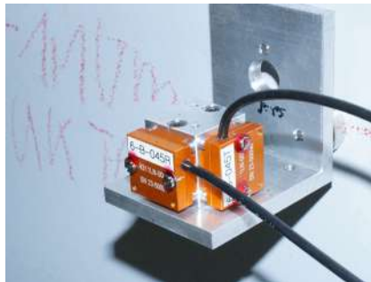
Measuring the vibrations of the tower induced by wind loading using biaxial acceleration sensors
