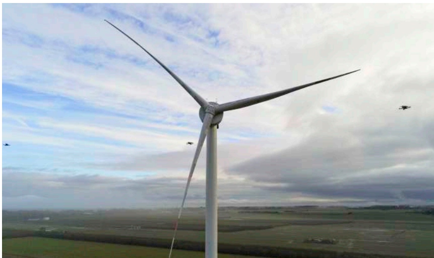
Drone fleet measuring the wake in front of the wind turbine OPUS 2
