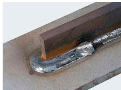
Top: Welded sample with test seam. Bottom: Fatigue fracture at the weld seam transition; the dot pattern is used for deformation measurement.
