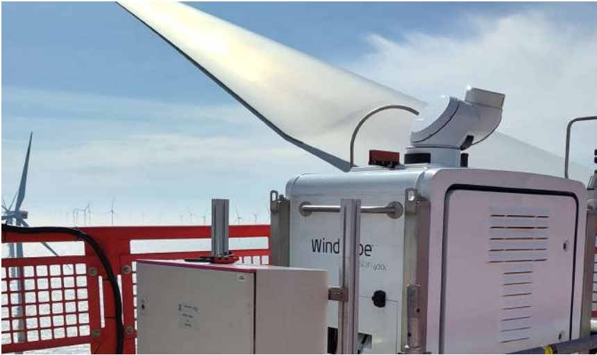
Scanning Lidar device on the nacelle of a wind turbine at RWE's offshore wind farm Amrumbank West. © Jörg Schneemann [2024]
