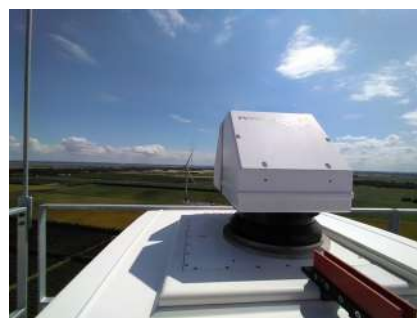
Gondola-mounted lidar on the wind turbine OPUS 1
