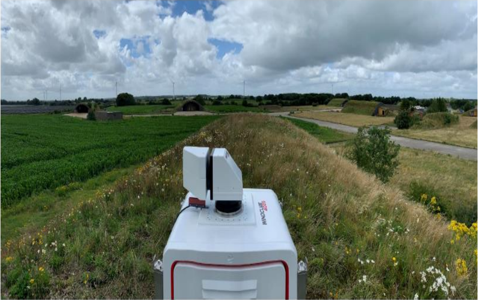
Figure 4: WLS400S- installed at DNV GL scanning lidar test pad.
