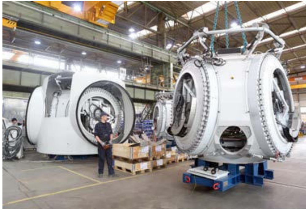
Production of nacelles at the Nordex DMR plant in Rostock Photo: Ove Arscholl
